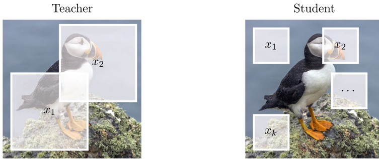
Fig. 11 Two sets of augmented crops for the teacher and student as defined by the multi-crop augmentation strategy. The teacher set contains two global views which cover at least 50% of the augmented image. The student set is made up of k patches that cover less than 50% of the other augmented version of the input image
